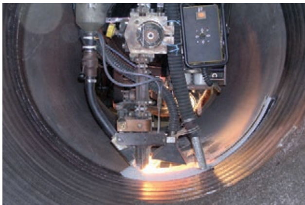
Strip cladding: BF 44/BA-Strip 309LN/Size: 60 x 0.5 mm
