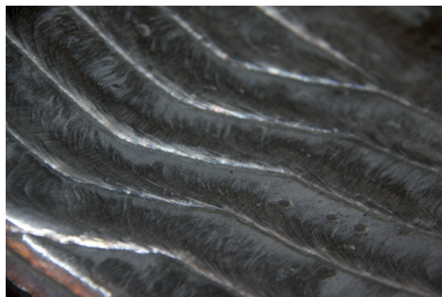
Strip cladding: BF 46/BA-Strip 625/Size: 60 x 0.5 mm (picture 1) and 30 x 0.5 mm (picture 2)
