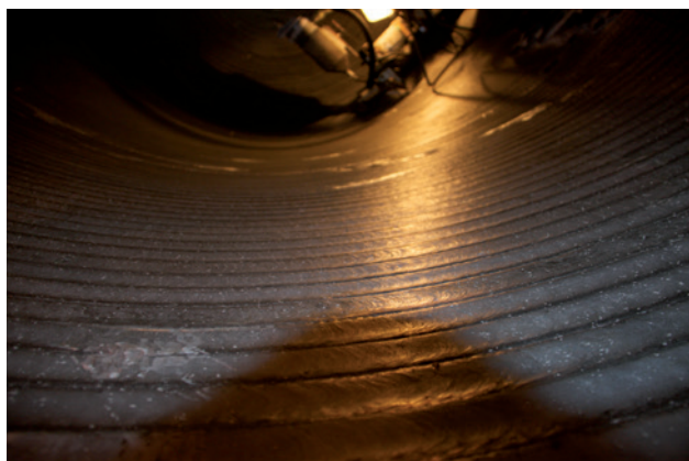
Strip cladding: BF 46/BA-Strip 625/Size: 60 x 0.5 mm (picture 1) and 30 x 0.5 mm (picture 2)
